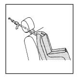
If the position you are using has an adjustable head restraint and you are using a single tether, raise the head restraint and route the tether under the head restraint and in between the head restraint posts.
